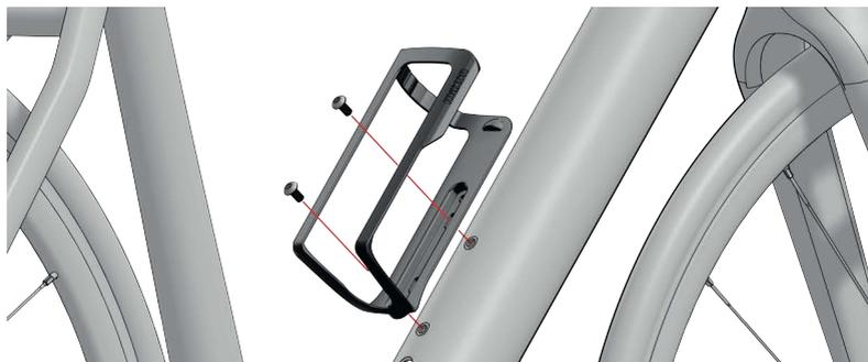
Figure 3-12 BIKEDRIVE AIR | Montage du support Range Extender
