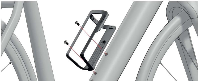
Abbildung 3-12 BIKEDRIVE AIR | Montage Range Extender halter
